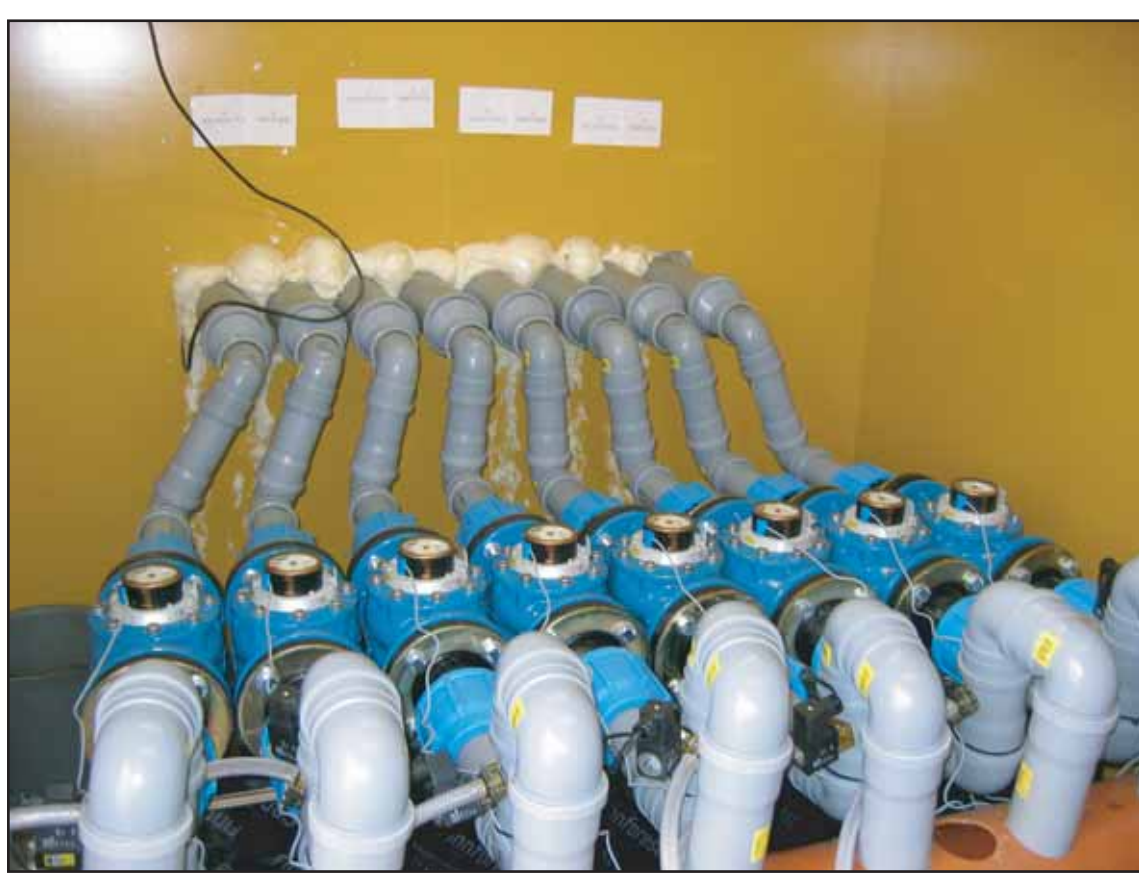
The subsurface and surface waters from each plot are measured. The flow-weighted water samples are collected through an electromagnet valve to plastic containers for further sampling and chemical analyses.
