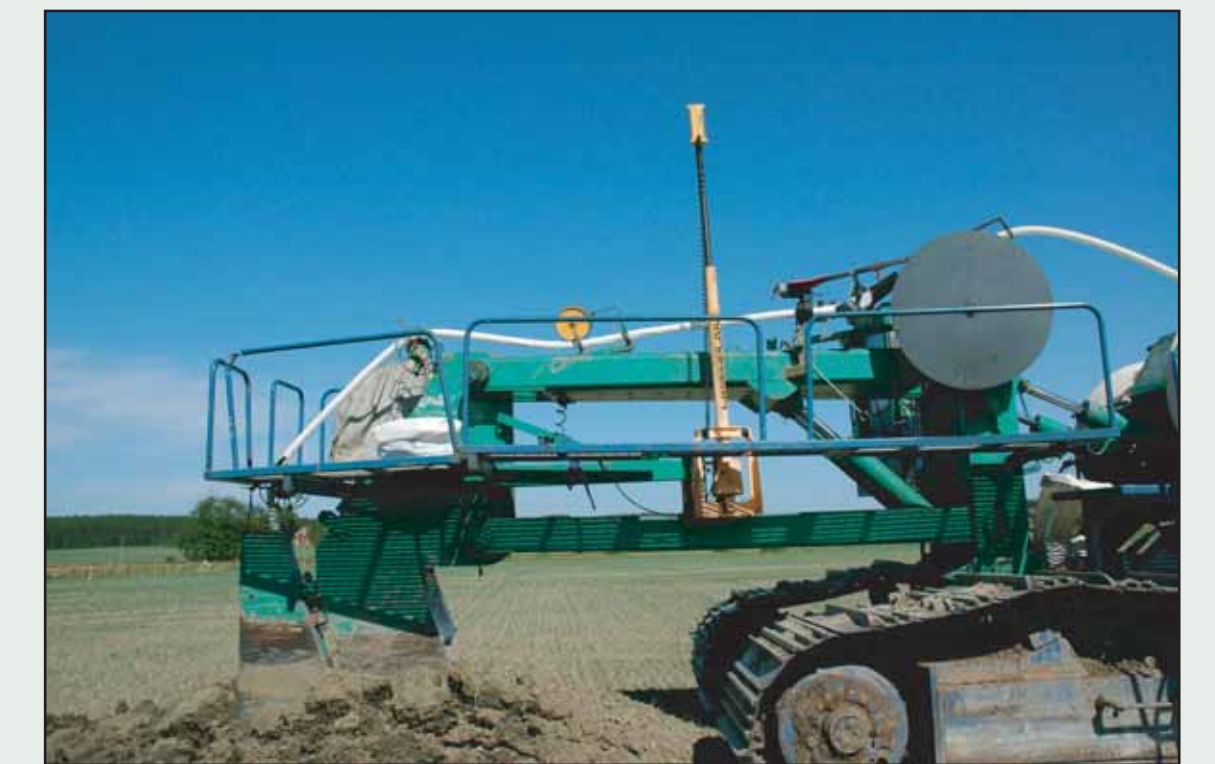
The drainage plow is equipped with a device that installs the envelope around the pipe on site before laying the pipe.
